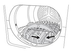
2. Lift slightly rack and take it carefully out from the drum.
